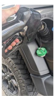
THE DESIGN OF THE ADAPTER ALLOWS THE SYPHON SHUTOFF ON THE FILL NOZZLE TO FUNCTION. IF THERE IS TOO MUCH FLOW, THE SHUT OFF WILL ENGAGE AND THE USER MUST REENGAGE THE FUEL FLOW.
